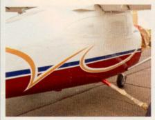
paint scheme. Having the longer final cure time also allows the last, clearcoat finish to bond properly to the paint layers beneath.
